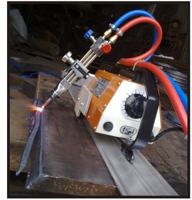
Bevel Cutting upto 45 Degree
